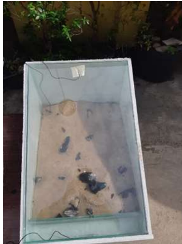
Gambar 3. Basin Tanpa Panel Solar Collector
