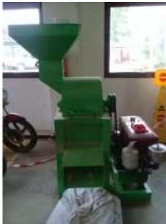
**Gambar 2.** Mesin Hammer Mill
