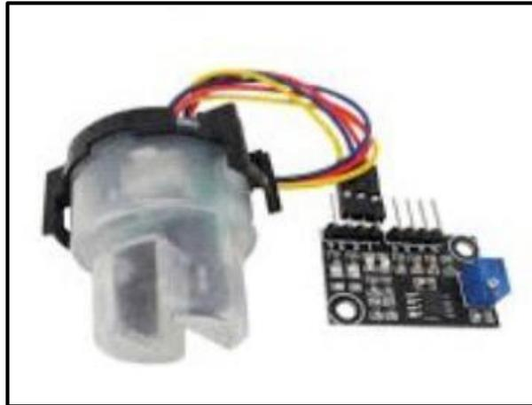
Gambar 1. *Turbidity Sensor Module* (Sumber: Wadu, 2017)
