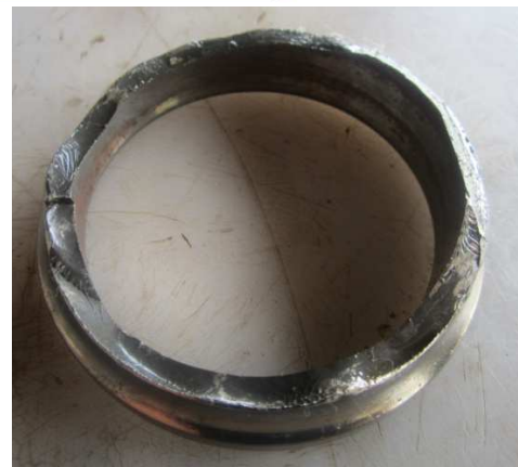
Gambar 5. Anti friction bearing P/N. 2D-5658 was broken and many material piece of Ball Anti friction bearing at housing.
