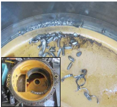
Gambar 5. Anti friction bearing P/N. 2D-5658 was broken and many material piece of Ball Anti friction bearing at housing.
