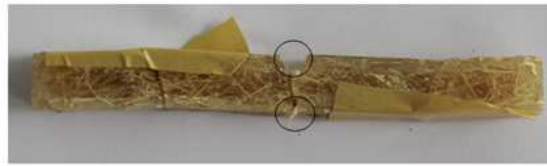
Gambar 5.3 patahan serat prosentase 45%
